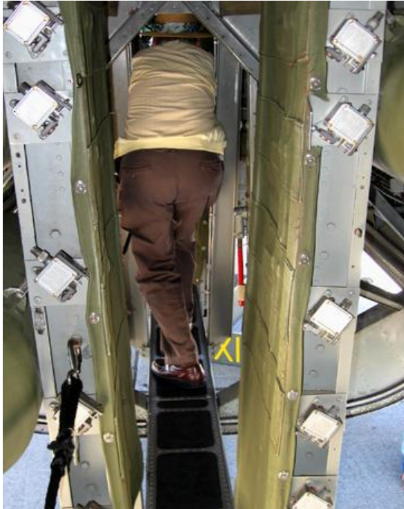
The 9 inch Catwalk in the Bomb Bay
